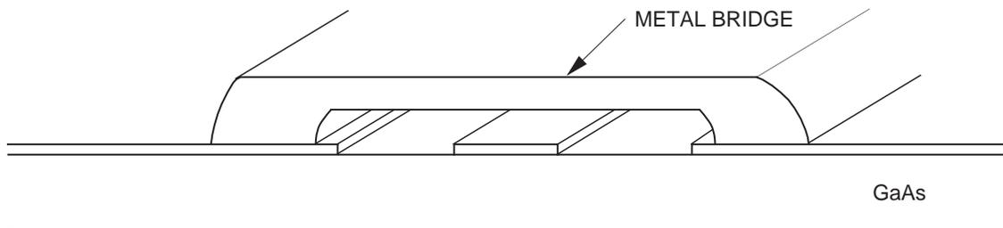
**Figure 3-28. Air bridge connecting coplanar waveguide ground planes.**
