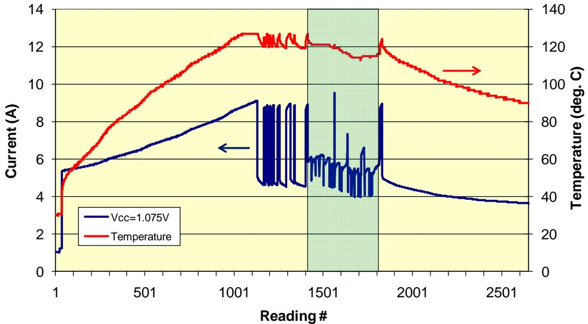
**Figure 1c.** Current and temperature for s/n:514 during latchup testing: angle=50 degrees, fluence = $2.0 \times 10^7$  gold ions per sq.cm, effective LET=145.5 MeV per mg/cm<sup>2</sup>
