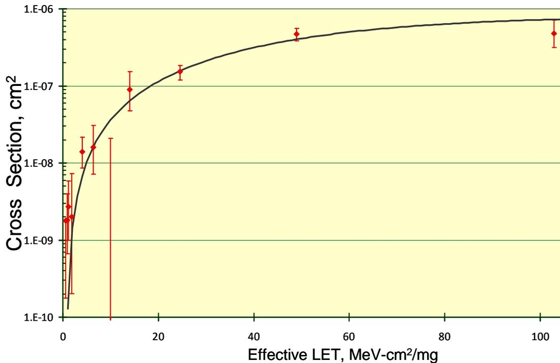
**Figure 4a.** Virtex-5QV SEFI Susceptibility due to Heavy Ion Strikes
