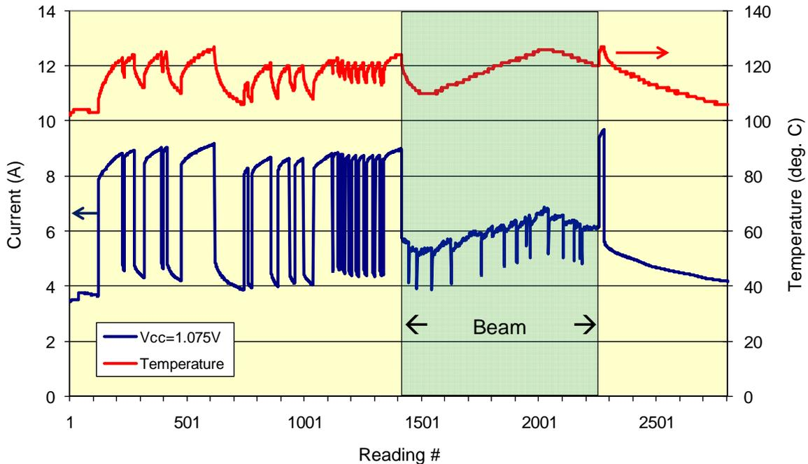
**Figure 1a.** Current and temperature for s/n: 592 during latchup testing: angle=50 degrees, fluence = $2.0 \times 10^7$  gold ions per sq.cm, effective LET=135.7 MeV per mg/cm<sup>2</sup>
