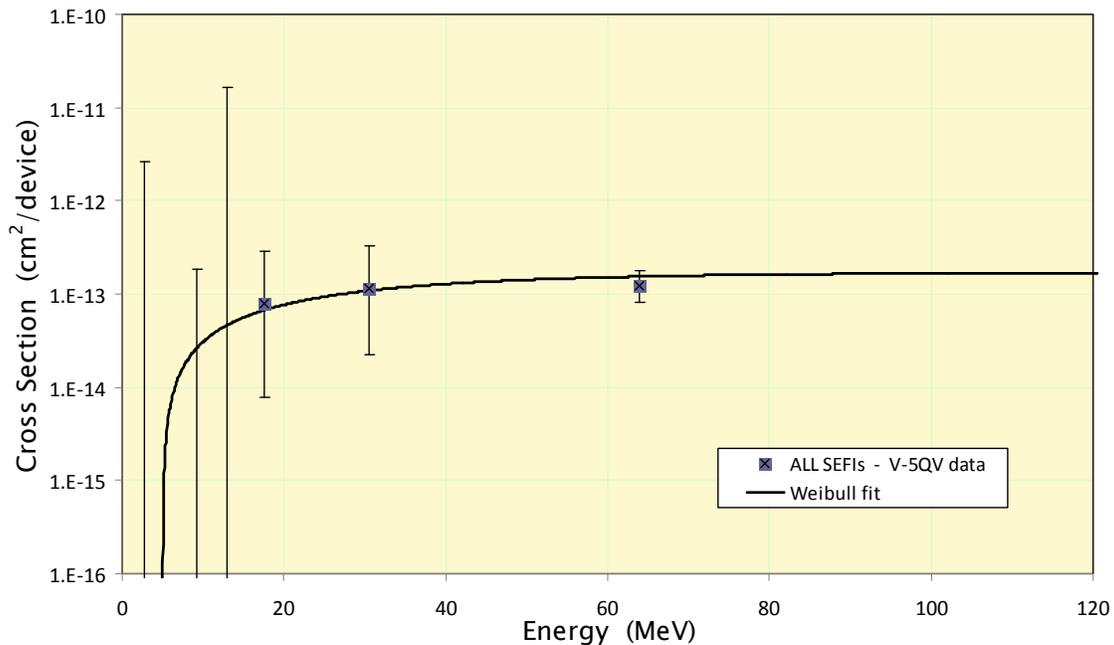
**Figure 4b.** Virtex-5QV SEFI Susceptibility due to Protons
