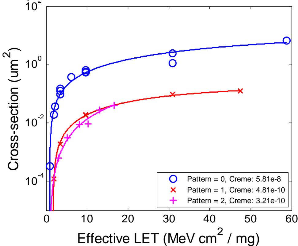
Figure 7. Virtex-5QV User Flip-Flop (with filters OFF) Susceptibility to Heavy Ions
