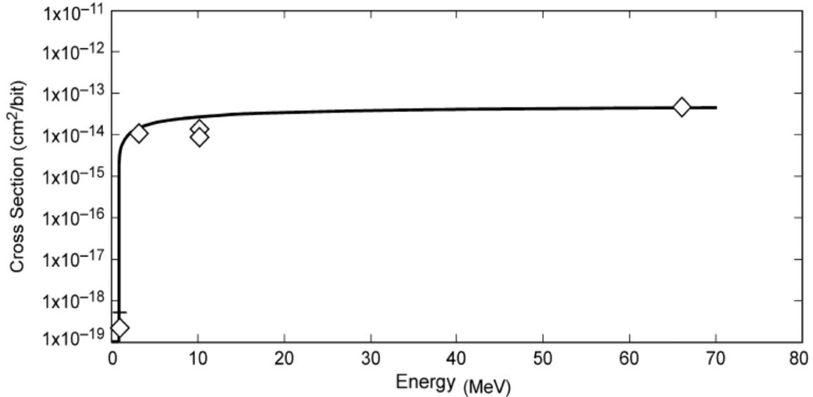
**Figure 6.** Virtex-5QV BRAM Susceptibility due to Proton Strikes
