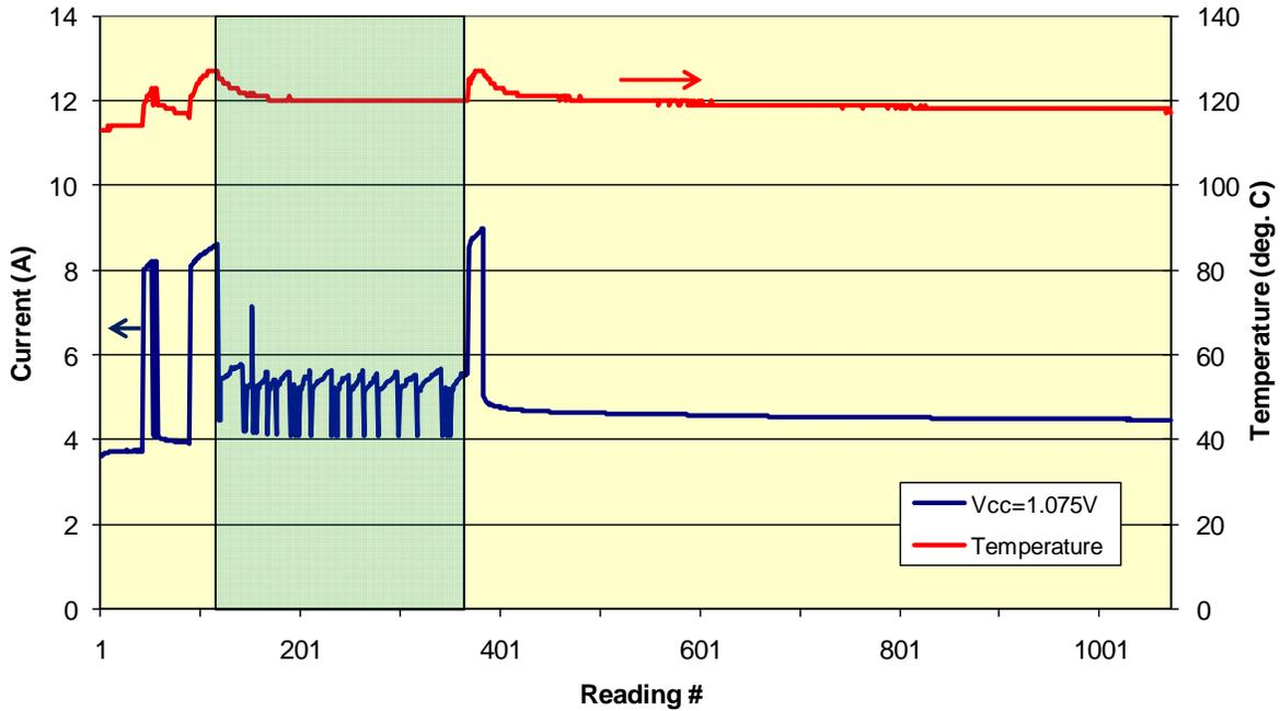
**Figure 1b.** Current and temperature for s/n:515 during latchup testing: angle=50 degrees, fluence = $2.0 \times 10^7$  gold ions per sq.cm, effective LET=145.2 MeV per mg/cm<sup>2</sup>
