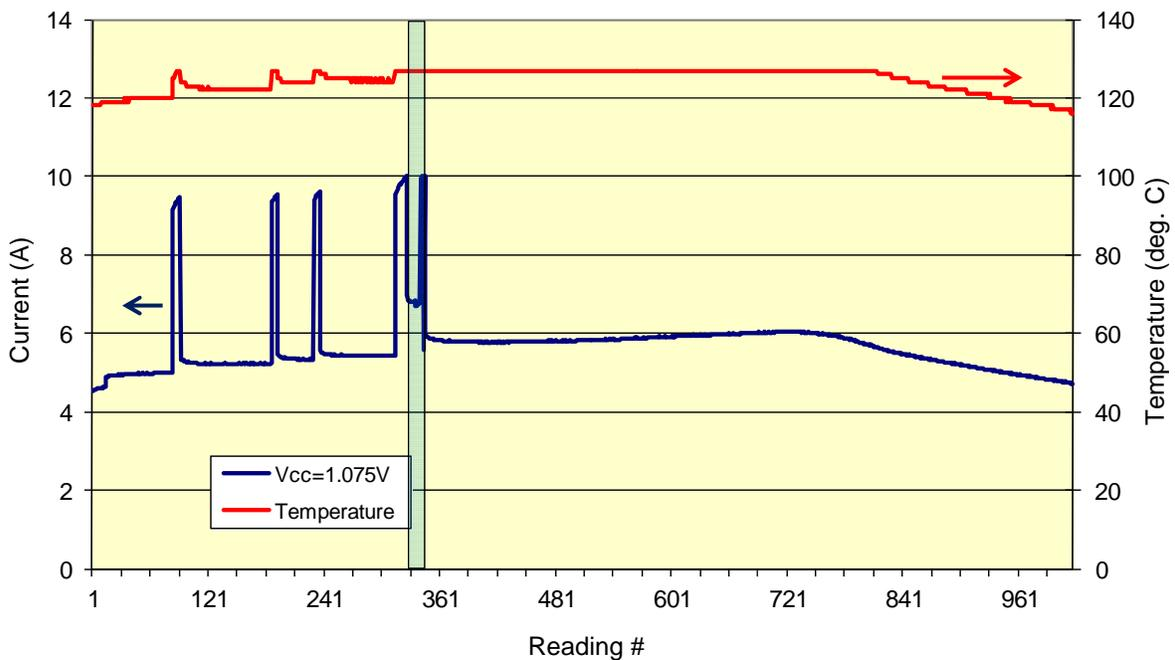
**Figure 2.** Current and temperature for s/n: 592 during latchup testing: angle=50 degrees, fluence  $< 2.8 \times 10^5$  gold ions per sq.cm, effective LET=135.7 MeV per mg/cm<sup>2</sup>
