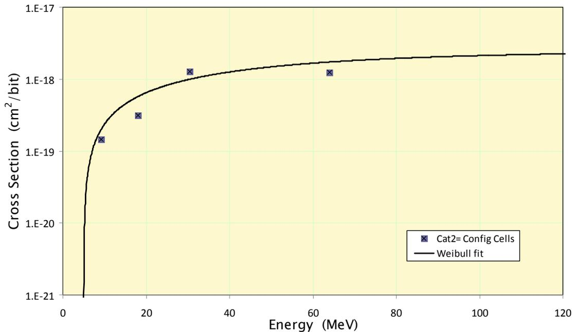
**Figure 11.** Virtex-5QV Configuration Bit Upset Susceptibility due to Protons
