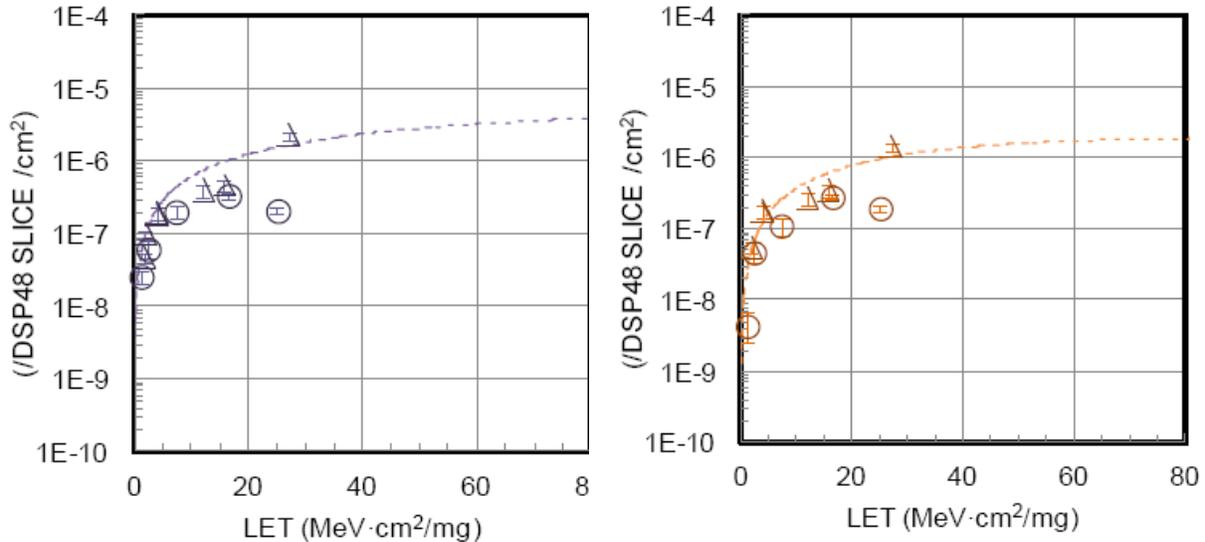
**Figure 8.** Virtex-5QV DSP Register(left= M, right=others) Susceptibility to Heavy Ions
