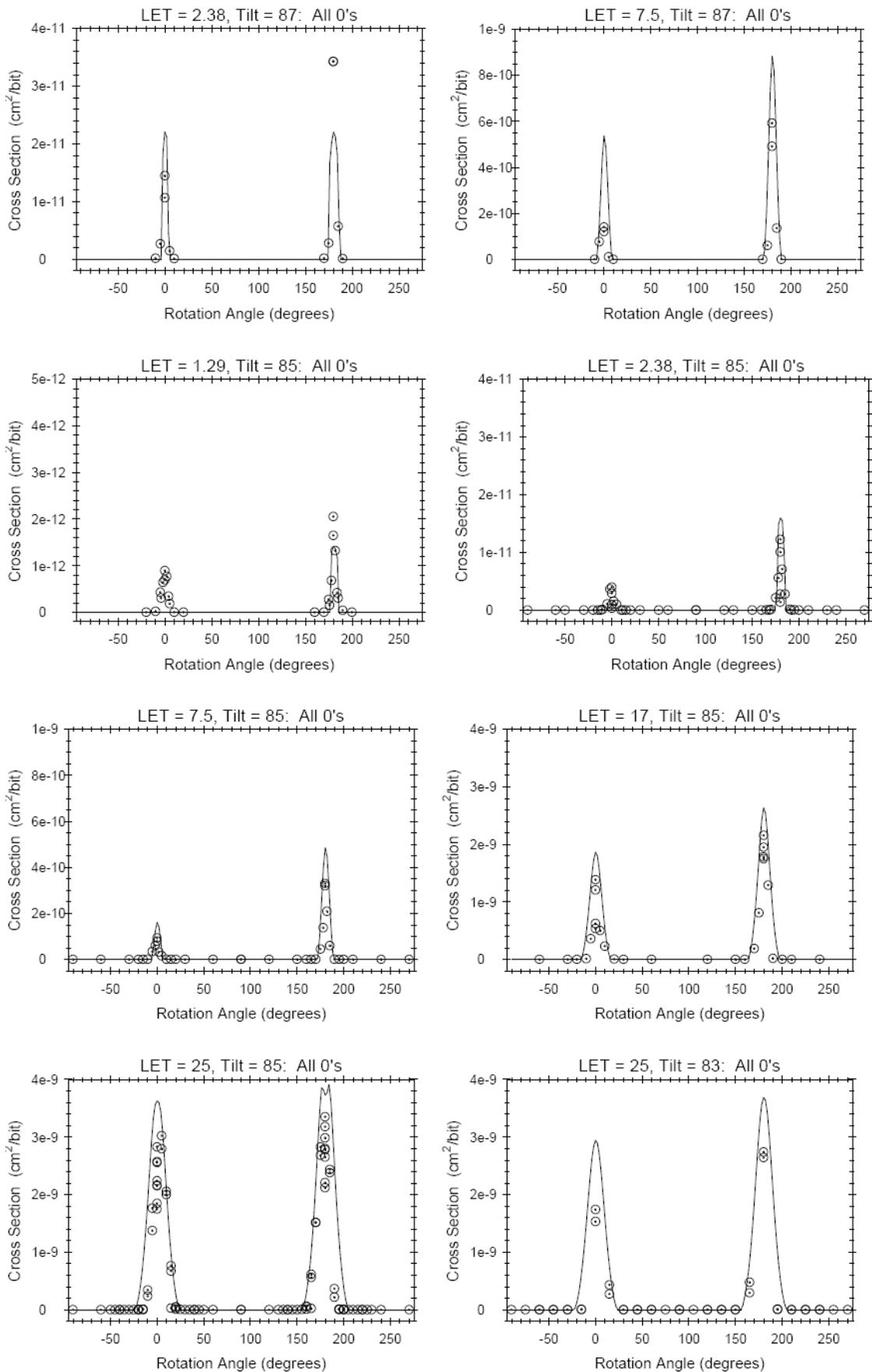
Fig. 10a. Rotation sweeps for dual-node the configuration cell storing zeros [from Ref.10, Fig.28 pt.1]
